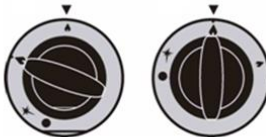
Figure1. Flame regulation with the gas tap – economy flame/maximum flame.
